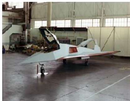
Fig A-11. Lockheed Martin built the “Have Blue” F-117 prototype for DARPA in the 1970s.
