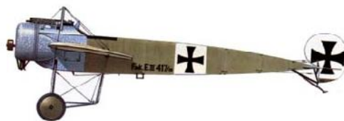
Fig A-7. The Fokker Eindecker III monoplane was fitted with an interrupter gear (synchronizer) which enabled a machine gun to fire through the spinning propeller
