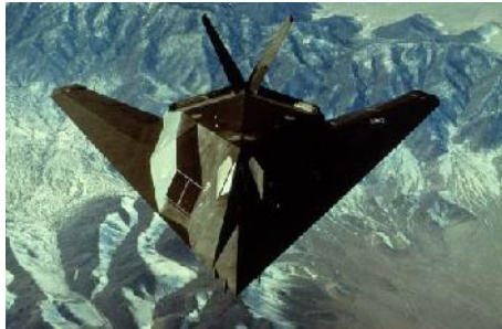
Fig A-12. The U.S. Air Force F-117A Nighthawk aircraft is the world's first operational aircraft designed to exploit low-observable stealth technology.
