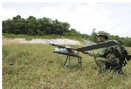
Fig B-3. An SAF scout trooper preparing to launch the Skyblade III mini-UAV
