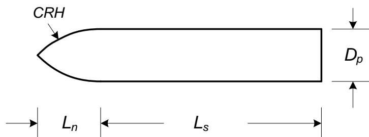
Figure 6.1 A typical ogive-nose projectile geometry (CRH - caliber-radius-head).
