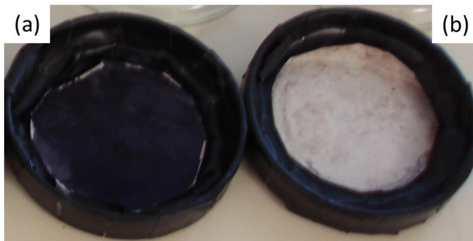
Figure 4.7. Pictorial view of a) membrane wetted with ethanol, b) membrane without ethanol wetting
