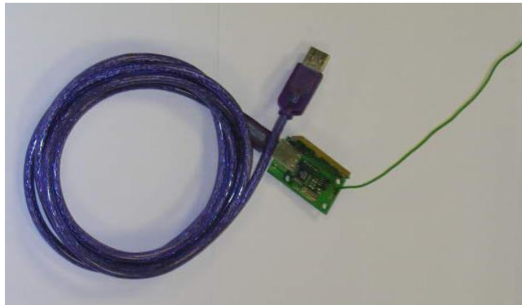
Figure 1.3: USB interface RF module on the workstation side.
