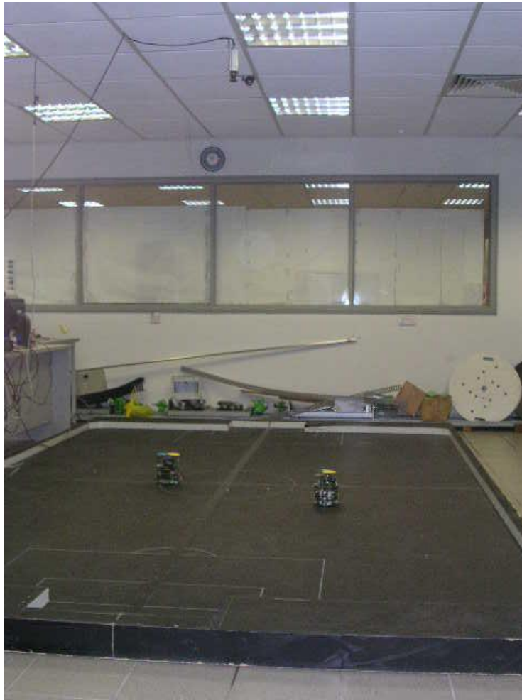
Figure 4.23: Picture of real robots, test bed(on the floor), CCD color camera with wide-angle lens and one web-cam(mounted on the ceiling).
