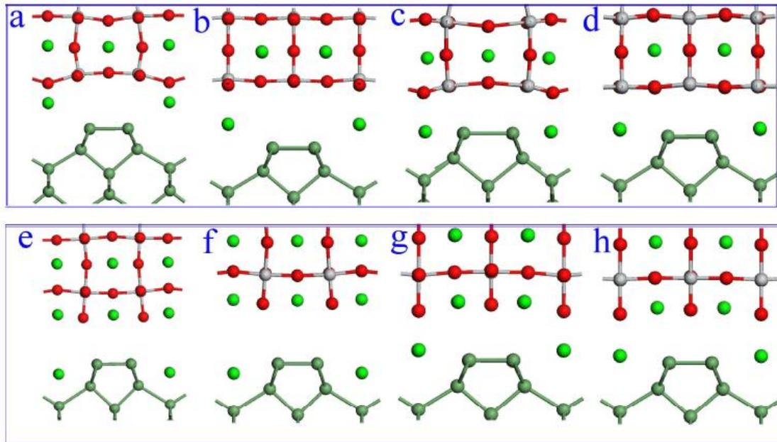
Figure 4.4. Interface structures for STO on Ge passivated by a Sr atom
