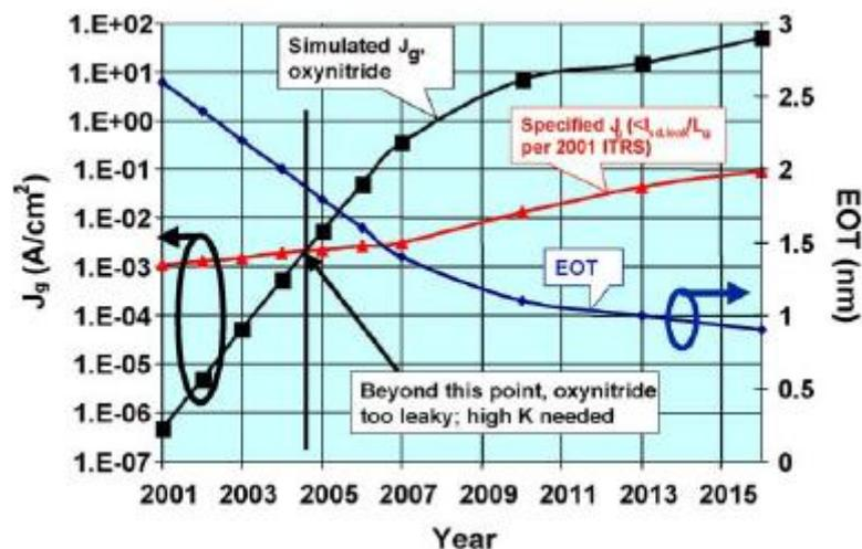
Figure 1.5. Gate leakage current, J<sub>g</sub> (SiON-based devices), and equivalent oxide thickness (EOT) of CMOS technologies, vs. the expected production year of these technologies. When the leakage current flowing through the SiON layer exceeds the ITRS requirements (here for low stand-by power technologies), an alternative gate dielectric should be used.
