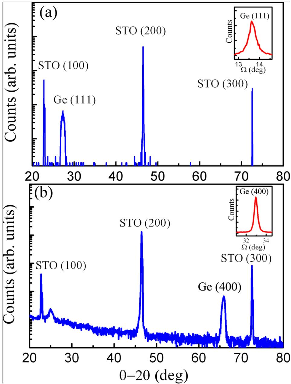
Figure 3.1. XRD  $\theta$ - $2\theta$  scan of Ge films deposited on STO (100) at temperatures of (a) 500 °C and (b) 650 °C, respectively. The insets show the  $\omega$  peaks of (b) Ge (111) and Ge (400) peaks, respectively.
