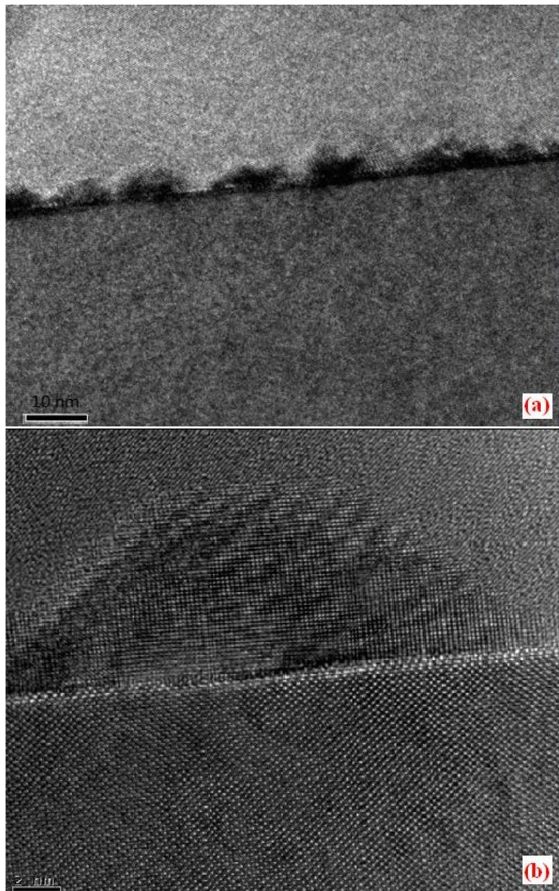
Figure 3.6. Cross section HRTEM images of the Ge films deposited on STO (100) at the substrate temperature of 650 °C for 6 mins: (a) 10nm scale, (b) 2nm scale
