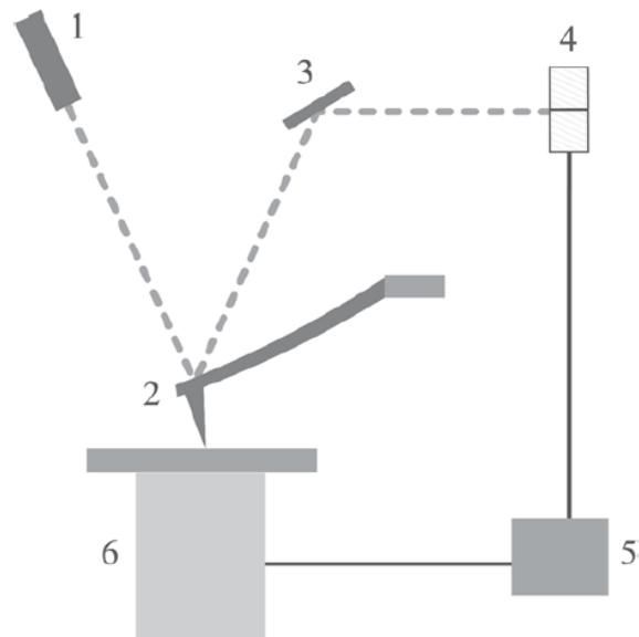
Figure 2.8. Schematic diagram of a scanned-sample AFM [10]
