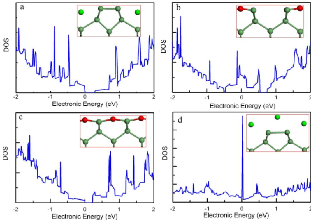
Figure 4.2. Total DOS of Ge surface passivated by a Sr atom (a), a O atom (b), two O atoms (c), and two Sr atoms (d) (the insets are the corresponding atomic structures).
