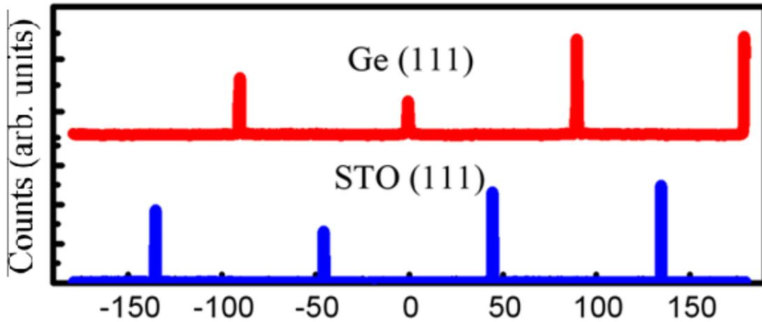
Figure 3.2. XRD phi ( $\Phi$ ) scans of Ge (111) plane and STO (111) plane for Ge sputtered on STO (100) at 500 °C
