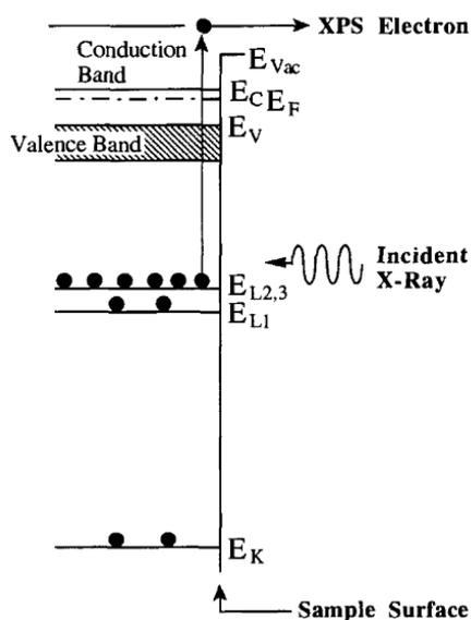
Figure 2.6. Electronic processes in X-ray photoelectron spectroscopy [9]
