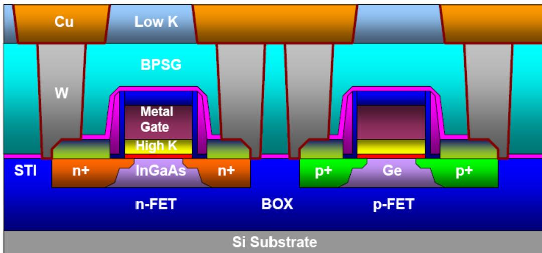
Figure 1.4. A schematic showing a possible combination of technology boosters. In the front end, device has high-k dielectric, metal gate electrode, and thin body, high mobility InGaAs for n-FET and Ge for p-FET. The back end interconnect includes low-k dielectric and low resistive metal Cu. [9]
