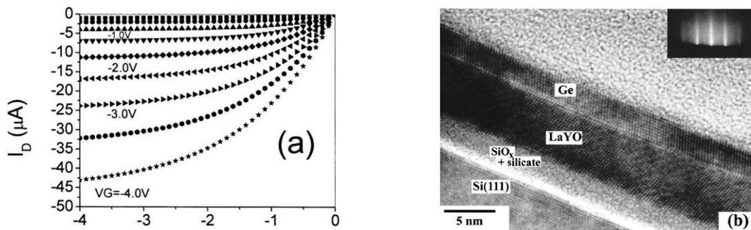
Figure 1.6. (a) the drain to source current ( $I_d$ ) plotted against the drain to source voltage ( $V_d$ ) as a function of different gate voltages ( $V_g$ ) in the GeOI-MOSFET; (b) high resolution transmission electron micrograph of an epitaxial Si(111)/LaYO/Ge structure.
