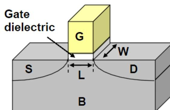
Figure 1.1. Schematic of a typical bulk MOSFET structure. Four terminals are denoted as Gate (G), Source (S), Drain (D), and Body (B). Geometry parameters are denoted as gate length (L) and gate width (w).
