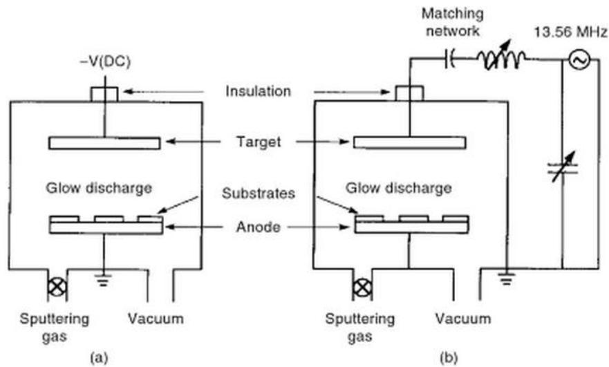
Figure 2.1. Schematic sputtering systems (a) DC and (b) RF [1]
