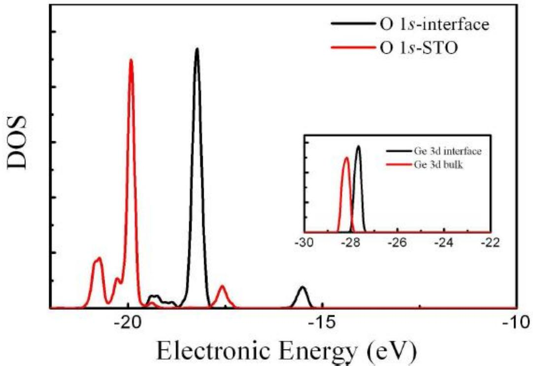
Figure 4.7. The rigid shift of O 1s and Ge 3d (inset) DOS between interface structure 3-c and the related bulk
