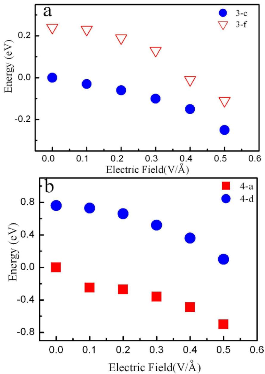
Figure 4.9. The dependence of interface stability on the external electric field: (a) interface structure 3-c and (b) interface structure 4-a.
