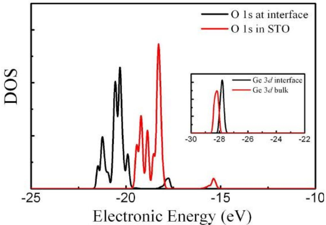
Figure 4.8. The rigid shift of O 1s and Ge 3d (inset) DOS between interface structure 4-a and the related bulk
