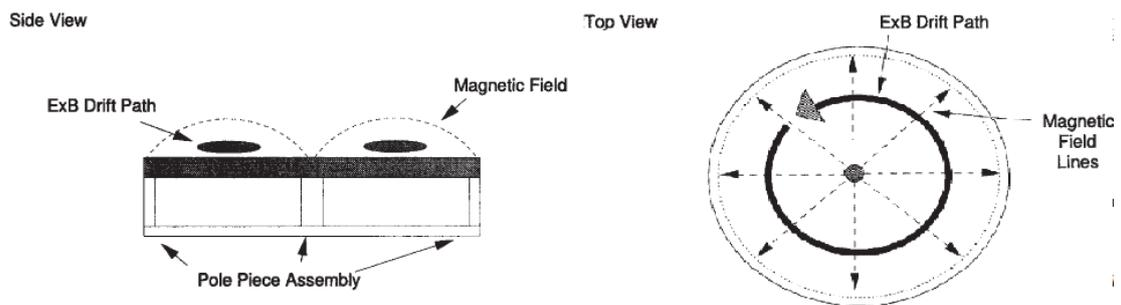
Figure 2.2. The magnetic field configuration for a circular planar magnetron cathode. [2]
