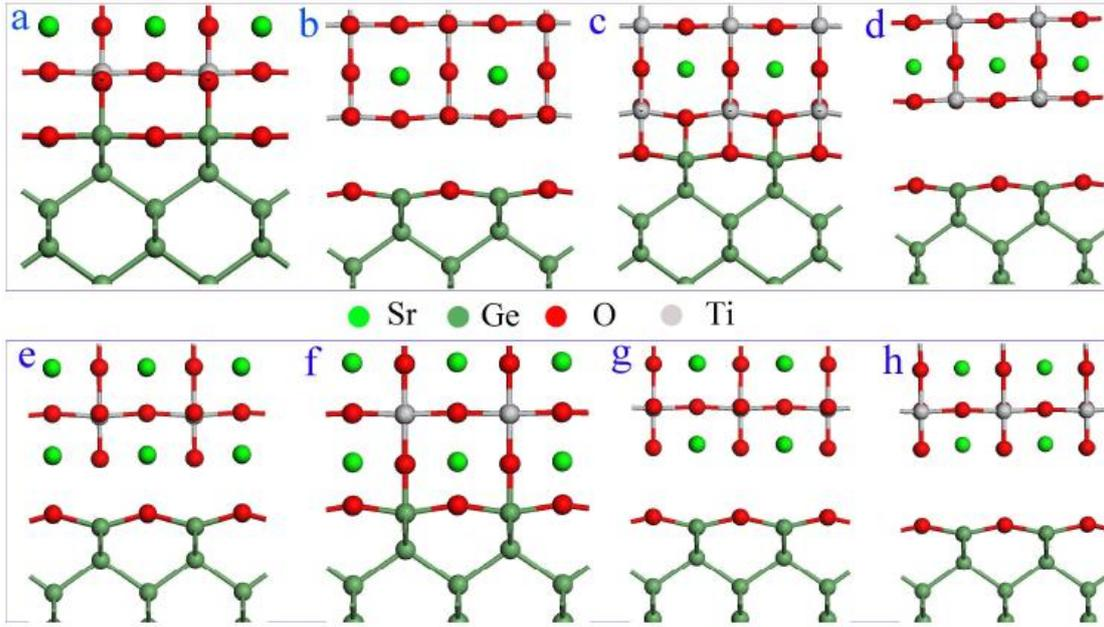
Figure 4.3. Interface structures for STO on Ge passivated by two O atoms
