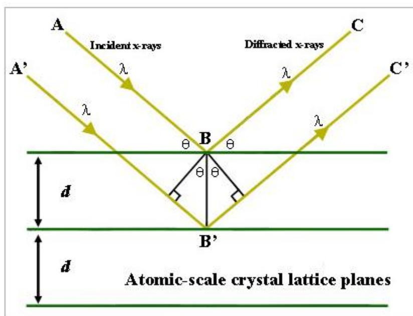
Figure 2.4. Bragg's Law reflection. The diffracted X-rays exhibit constructive interference when the distance between paths ABC and A'B'C' differs by an integer number of wavelengths ( $\lambda$ )
