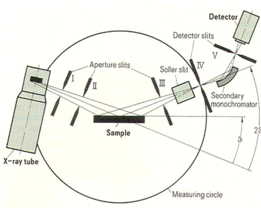
Figure 2.5. Schematic of a Powder X-ray diffractometers
