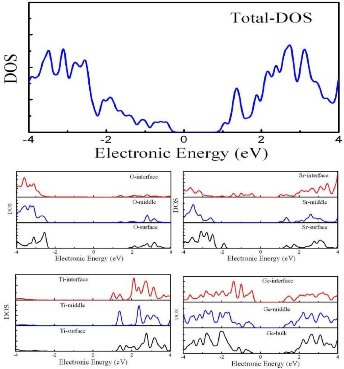
Figure 4.6. The total and projected DOS for the interface structure 4-a
