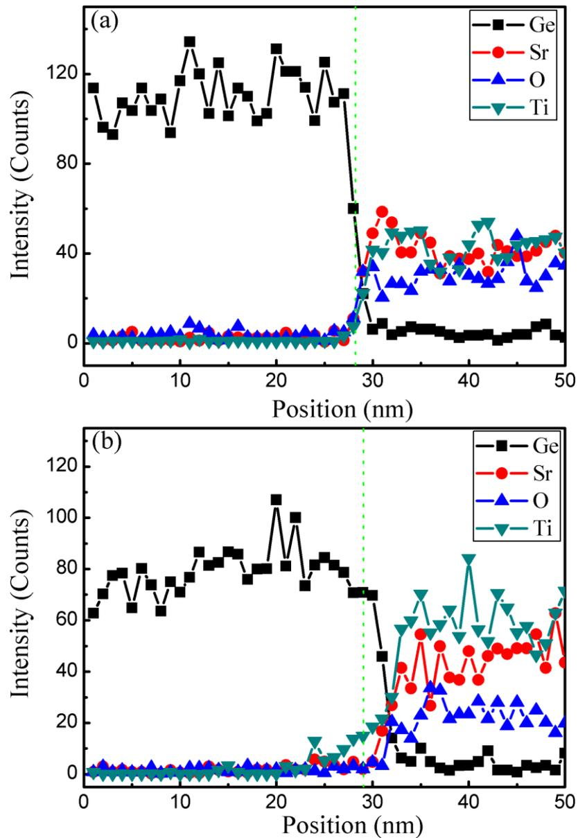
Figure 3.4. STEM EDX line-scan of interfacial chemical compositions for the Ge films on STO (100) at temperature of: (a) 500 °C and (b) 650 °C. The vertical line indicates the position of the Ge/STO interface.
