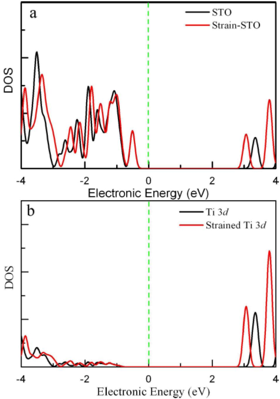
Figure 4.1. (a) Total DOS of STO with/without tensile strain. (b) Projected Ti 3d DOS of STO with and without strain.
