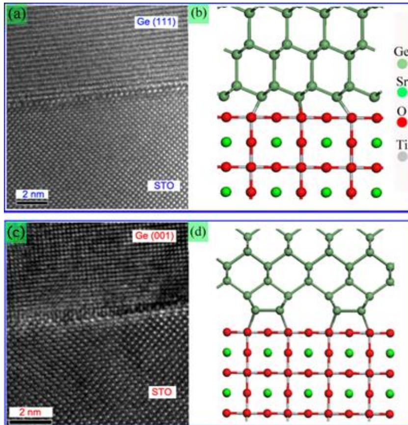
Figure 3.3. Cross section HRTEM images of the Ge films deposited on STO (100): (a) the formation of crystalline Ge (111) on STO (100) at the substrate temperature of 500 °C, (b) a schematic interfacial atomic structure for Ge (111)/STO (100), (c) the formation of crystalline Ge (001) on STO (100) at the substrate temperature of 650 °C, and (d) a schematic interfacial atomic structure for Ge (001)/STO (100).
