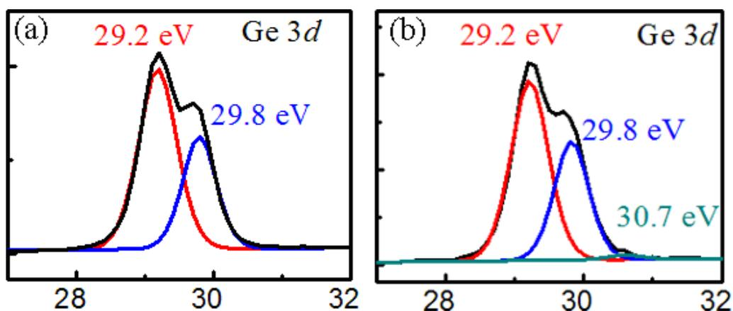
Figure 3.5. The XPS core-level spectra of Ge 3d for the Ge thin films grown on STO (100) with the deposition time of 6 mins and the substrate temperature of (a) 500 °C and (b) 650 °C.
