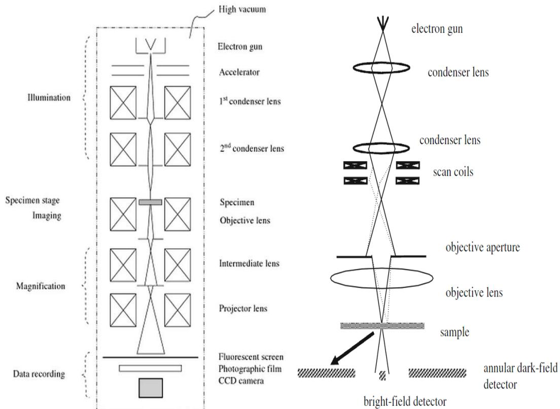
Figure 2.3. Schematic of TEM (left) and STEM (right) [3]
