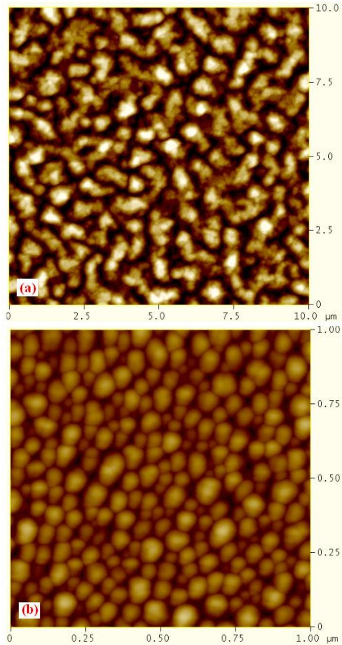
Figure 3.7. AFM images of the Ge films deposited on STO (100) at the substrate temperature of 500 °C for: (a) 60mins, (b) 6mins
