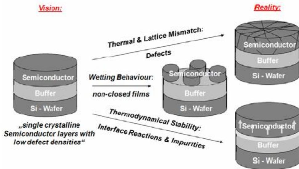
Figure 1.7. Overview of important epitaxy parameters to achieve the integration of high quality semiconductor layers via oxide heterostructures on Si.
