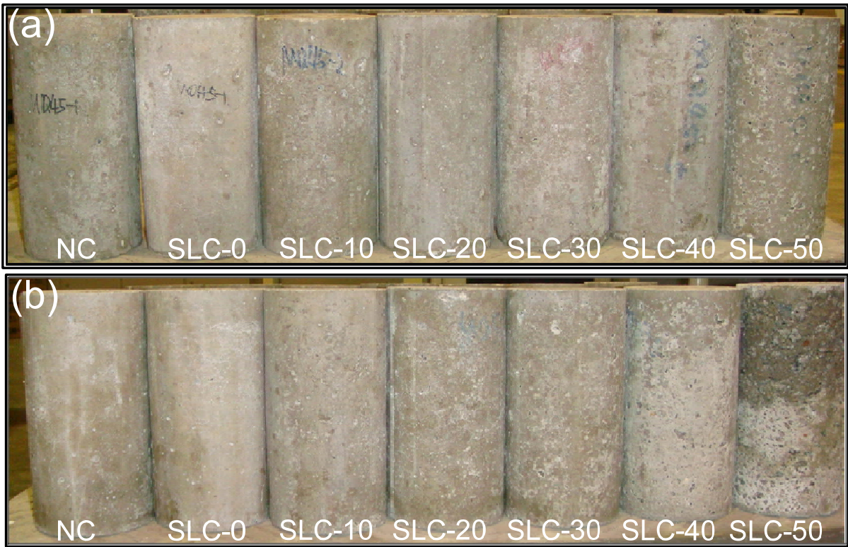
Figure 4-20: Pictures of “sandless concrete” after sulfate attacks with w/c ratio of (a) 0.45, and (b) 0.50.
