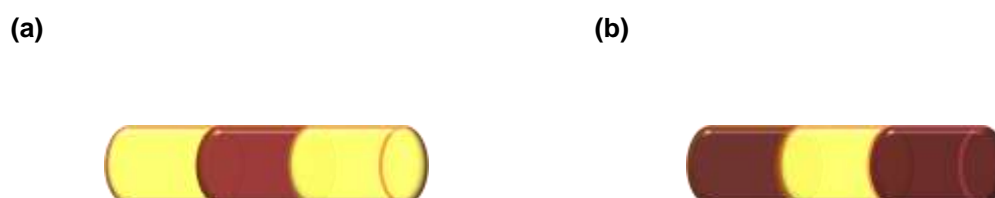
Figure 3.1. Cartoon illustration of (a) ABA and (b) BAB nanorods, where A denotes CdS and B denotes CdSe.
