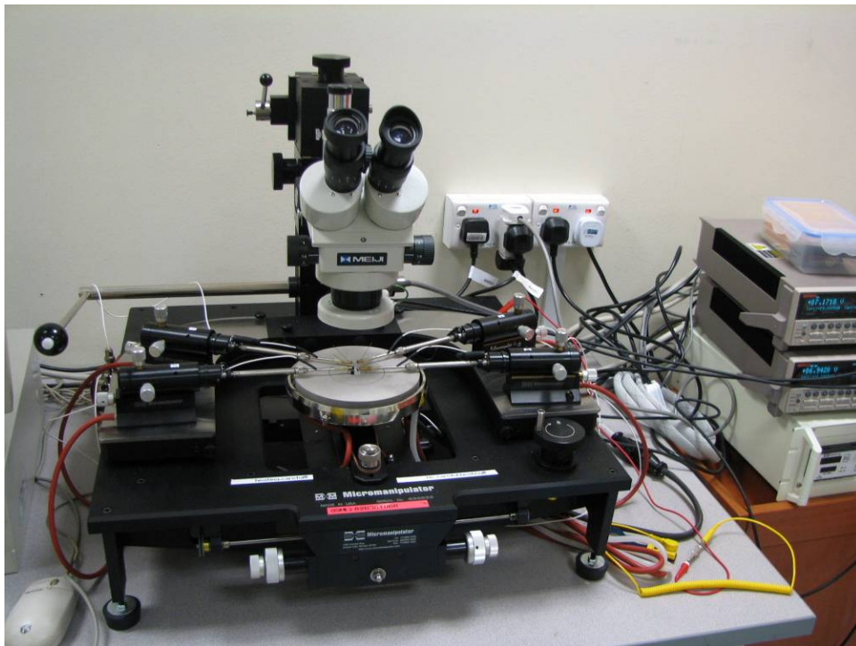
Fig. 3.5 Micromanipulator Probe Station used for measuring EM failure lifetimes.
