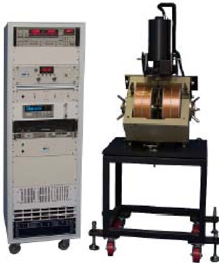
Fig. 3.10 Vibrating sample magnetometer (VSM) system used for measuring the magnetic properties.
