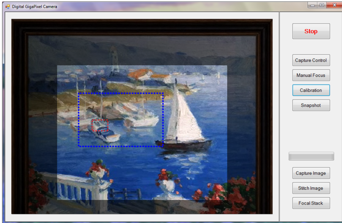
Figure A.13: You could select the region to be captured by clicking and dragging on the viewfinder in the main window. The region to be captured will be highlighted by a blue dashed rectangle.
