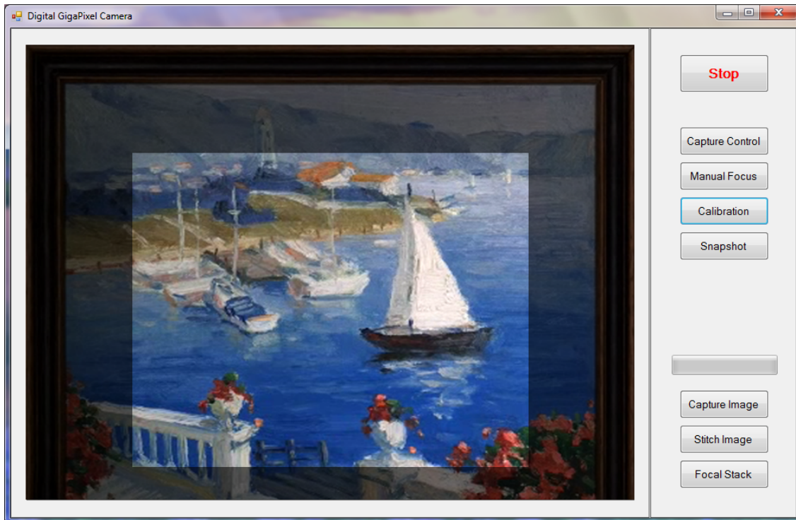
Figure 2.8: The main window contains a viewfinder on the left and a control panel on the right. Note the dimmed area is the scene that will not be captured by the camera.
