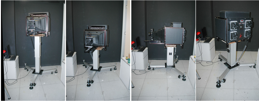
Figure 2.6: Camera pier. The camera is mounted on a telescope pier that allows adjusting the height of the camera. (Images courtesy of Moshe Ben-Ezra)
