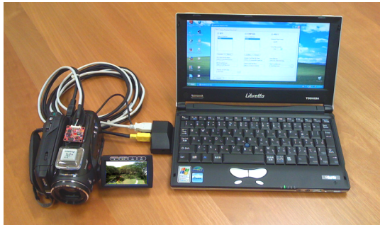
Figure 1.2: Early setup for geo-tagged video data collection: laptop computer, OceanServer OS5000-US compass, Canon VIXIA HV30 camera, and Pharos iGPS-500 receiver.
