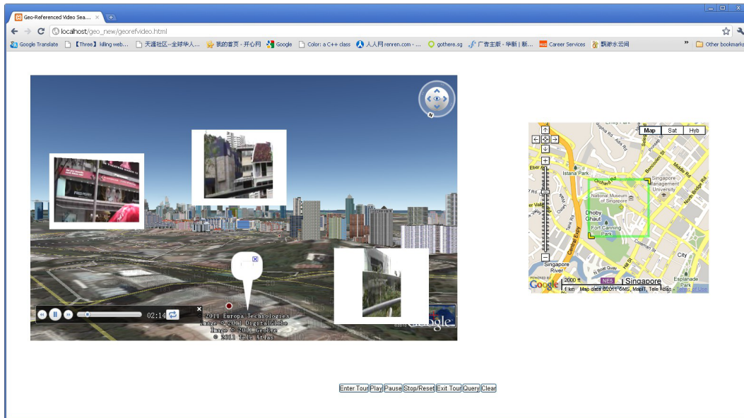
Figure 3.5: Geo-referenced 3D video search engine web interface showing multiple videos simultaneously.
