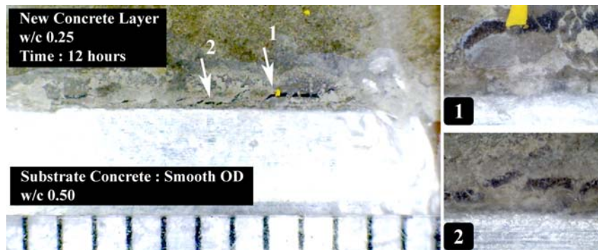
Figure 5.31 De-lamination at the interface of the unsealed composite specimen monitored from the side of the specimen at 12 hours after adding water to the mixture (OD substrate with smooth surface)
