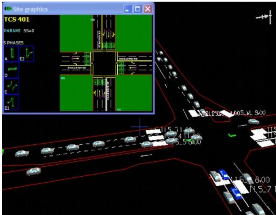
Figure 6.3. Snapshot of SCATS traffic controller and the controlled intersection
