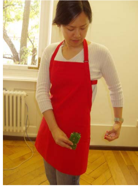
Fig. 1. (Left) The accelerometer is kept in a little pouch attached to the apron string located above the waist. Fig. 2. (Right) The base unit of fall detector (without casing in picture) is located at the lower pocket of the apron.
