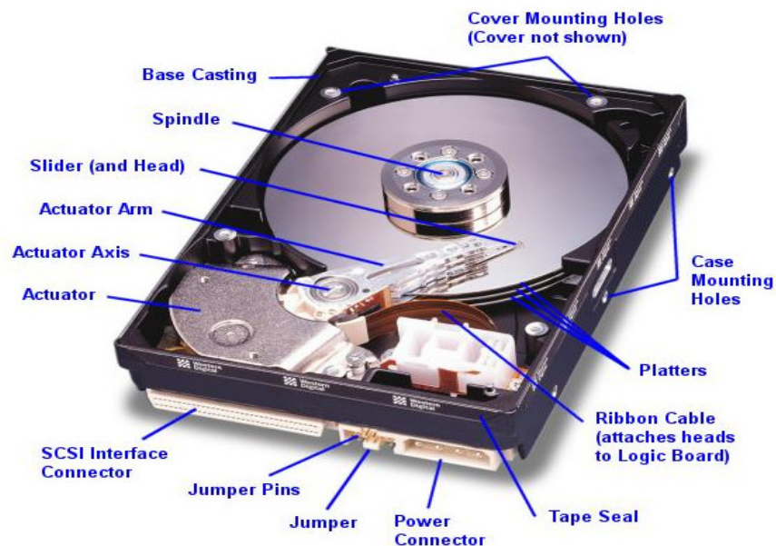
Figure 1.2 Components of a typical hard disk drive [4]
