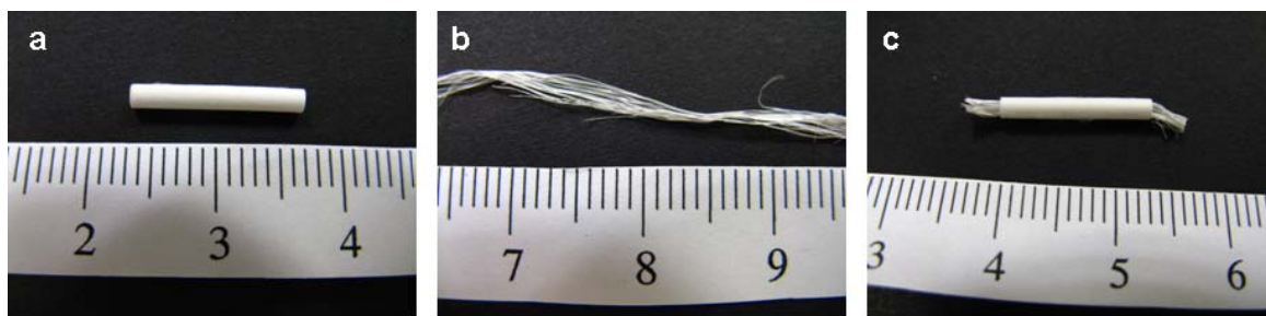
Figure 6.6. Macrographs of nanofibrous nerve construct. (a) bilayered nanofibers nerve conduit, (b) intra-luminal guidance channels, and (c) nerve conduit containing intra-luminal channels.
