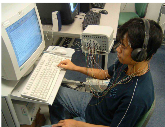
Figure 3.2: The experiment set-up for mental-fatigue EEG database collection.
