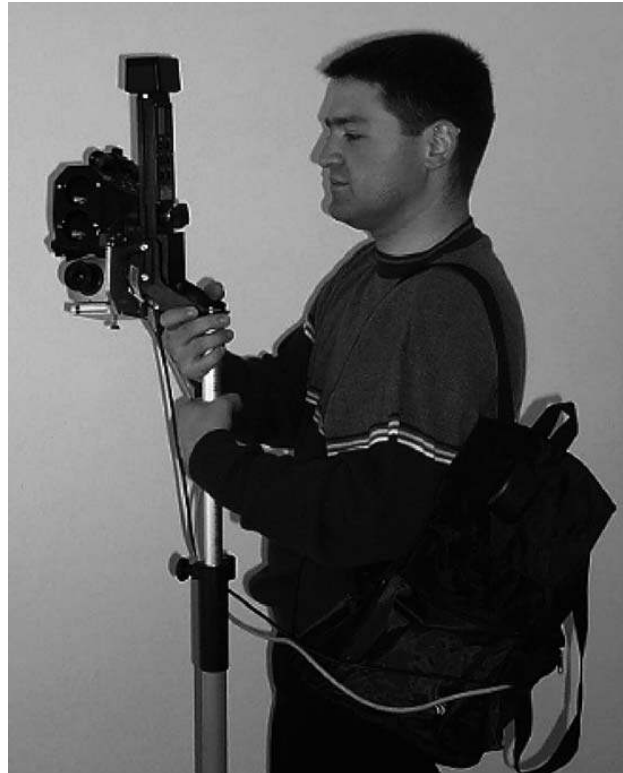
Figure 3.1: Prototype of direct referencing sensors rig (Haala and Bohm, 2003).
