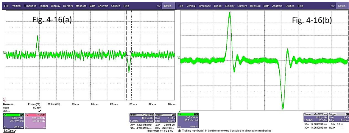
Figure 4-16(a): Velocity measurement 25mm/s/V, 5 \mu m, 250 RPM, 20 nm (left) Figure 4-16(b): Velocity measurement 5mm/s/V, 5 \mu m, 250 RPM, 20 nm (right)
