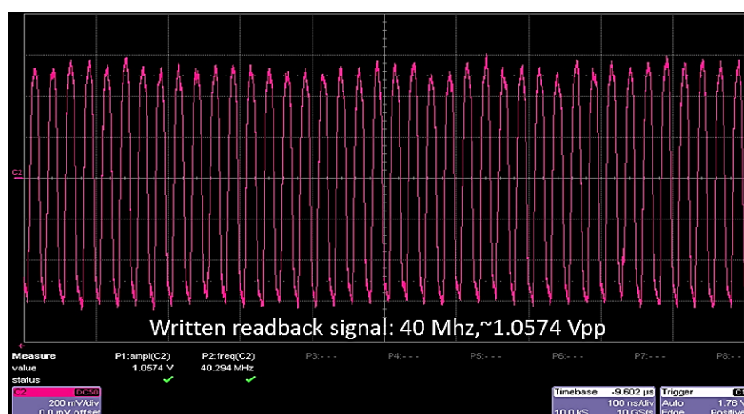
Figure 3-11: Overwritten data with 40 MHz all 1s pattern
