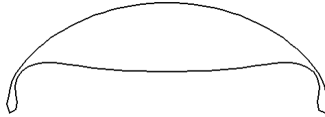
Fig. 3.19 The final collapsing shape of the 1 \mu\text{m} bubble as shown in Fig. 3.18. The bottom surface moves with high speed towards the upper surface (about 1000 m/s for this 1 \mu\text{m} bubble. Larger bubbles of radii 10 and 100 \mu\text{m} , collapse with jet speed of about 1000 and 500 m/s, respectively).
