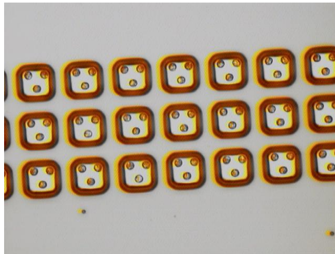
Fig. 3-11 Top view of solder plating window defined with THB110N
