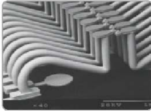
Fig. 2. 9 FormFactor's MicroSpring Contacts
