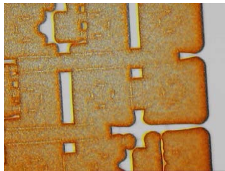
Fig. 3. 18 Enlarged Photos for Exposure 30seconds for the PR Patterning
