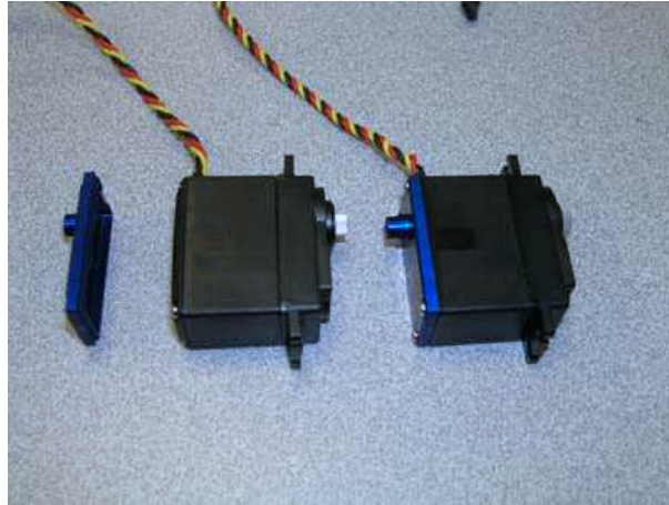
Figure 3.2: The motor cover, original motor and modified motor
