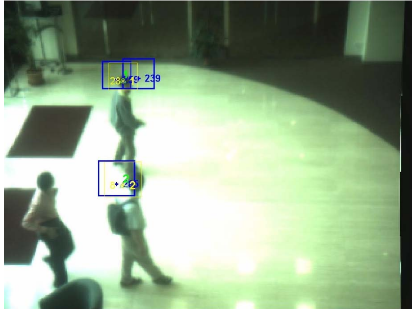
Figure 5.3 The tracking method leads to more accurate head position than the detection does (including one false alarm of detection method)
