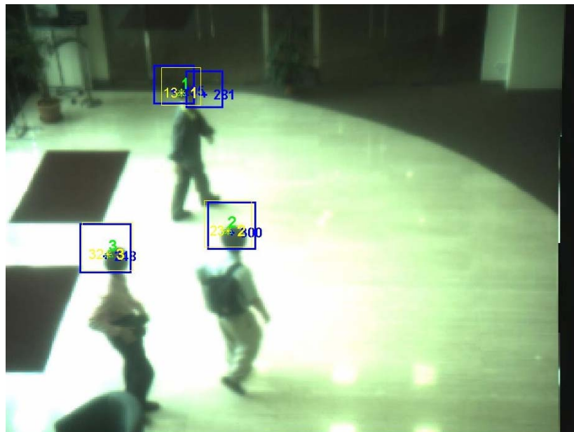
Figure 5.2 The false alarm in the detection result has been eliminated in the tracking result
