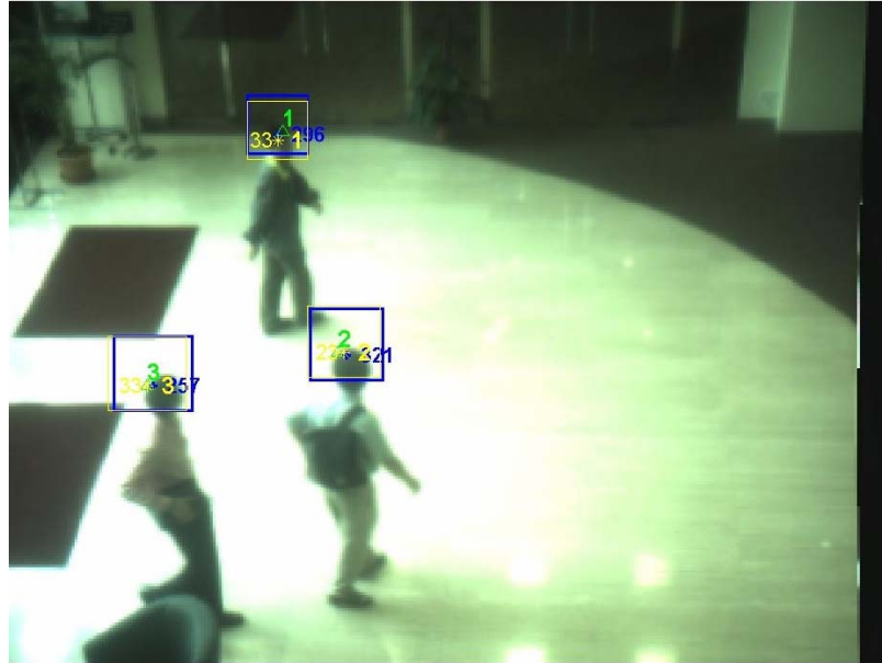
Figure 5.1 An example of tracking results (yellow) as well as detection results (blue)
