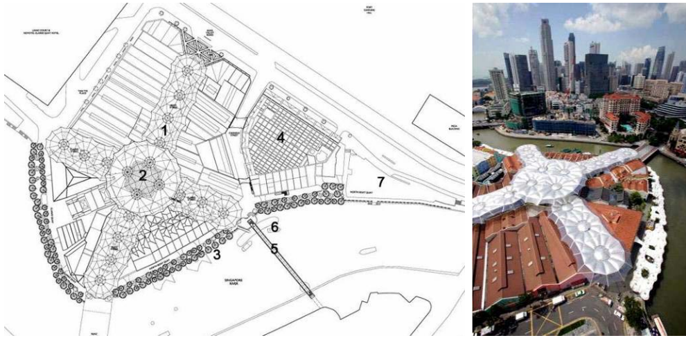
Figure 53 (left) the site plan of Clarke Quay: 1. “angel” canopy; 2. central fountain square; 3. “lilypad and bluebell” riverfront dining; 4. parking garage; 5. proposed pedestrian bridge; 6. river transport dock; 7. 24-hour G-max bungee ride (source: SMC Alsop with RSP Architects. "Clarke Quay Revival.", amended by the author); (right) aerial view of the new Clarke Quay (source: http://www.europaconcorsi.com/db/cache/pub/pub_13010_w500h500q75bw1_1435055803.jpg ).
