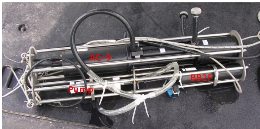
FIGURE 3.5: The Cage encasing the equipments
