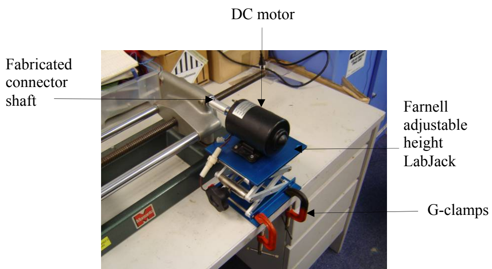
Fig. 30 Implementation of motor to automate drawing process.
