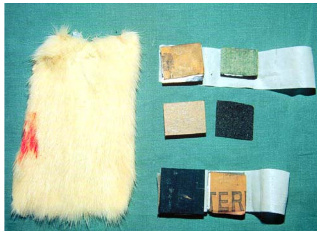
Fig. 3.7: Experimental set-up for biomechanical testing. Fresh skin for testing and sandpaper interfaces to enhance the gripping by the materials testing machine are seen in this picture
