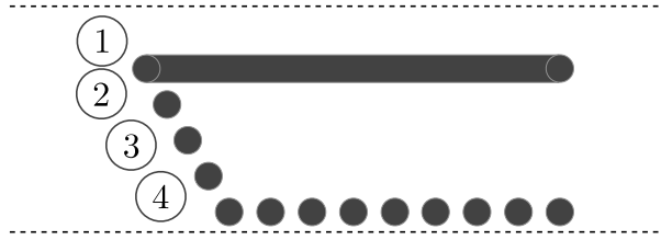
Figure 4.8: Position of fixed particles with radius \sigma = 1.8 \delta_p , that have been used to estimate the effect of finite-size particles on the asymmetry of the flow. The horizontal dashed lines indicate the extension of the unit cell in y -direction.
