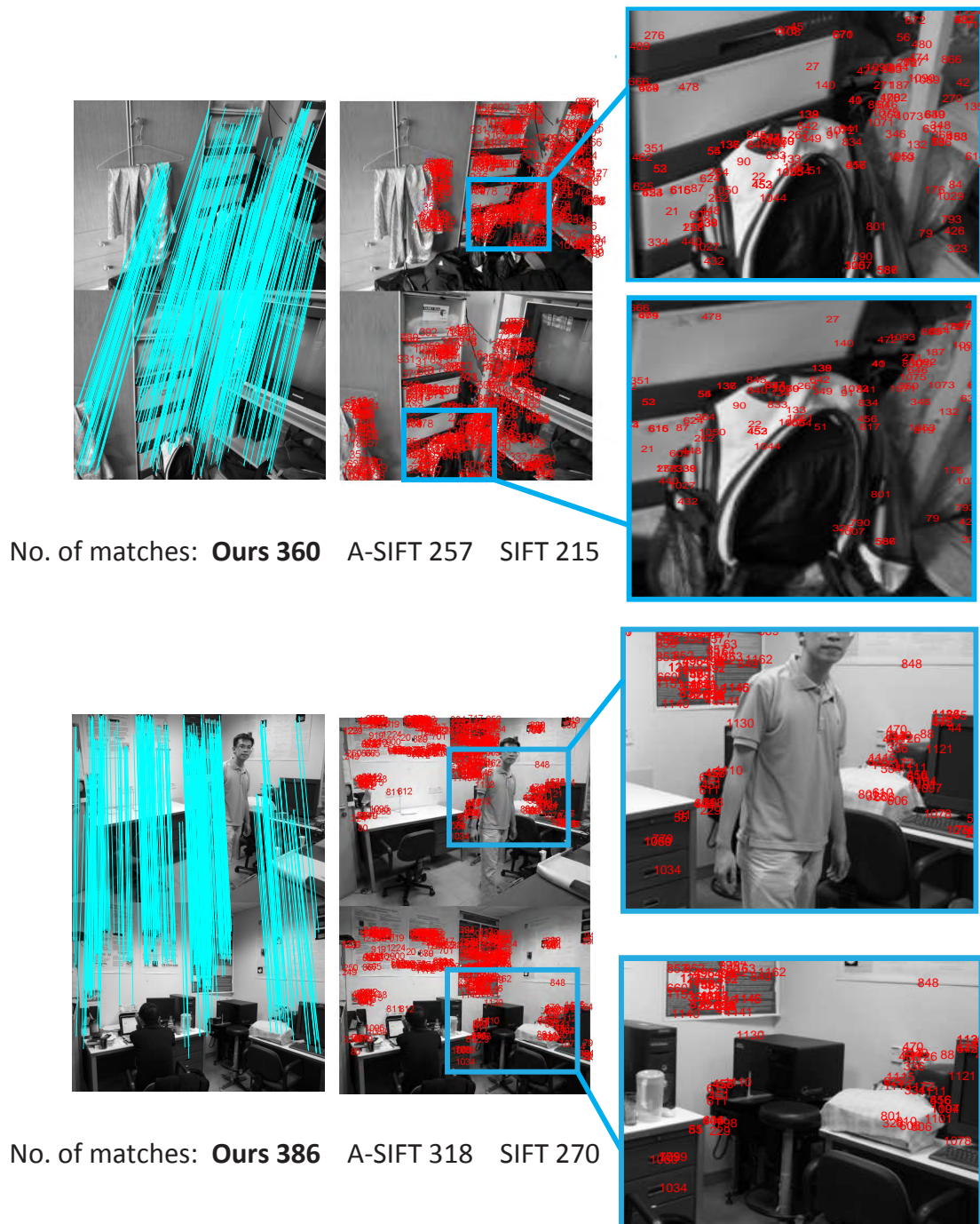
FIGURE 4.11: We show the results obtained by using our algorithm as a matcher and compare against conventional nearest neighbor SIFT [64] and A-SIFT [76] feature matching. Although we use traditional SIFT [64] descriptors, we can obtain more matches than applying nearest neighbor matching to the more sophisticated A-SIFT descriptor. The above figures shows that the additional matches do not come at the expense of accuracy and the matching is stable to significant occlusion.
