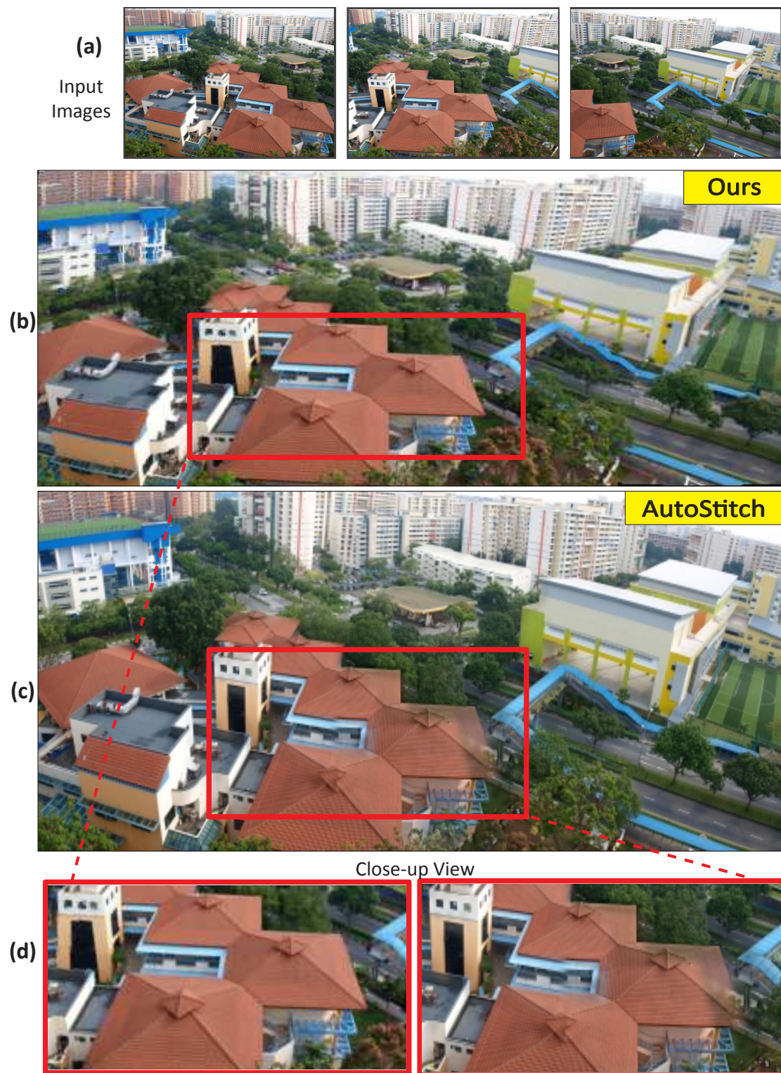
FIGURE 4.9: Input images in (a) are taken from a series of windows. Our mosaic in (b) is perceptually accurate while homographic mosaicing using AutoStitch [12] in (c) has difficulty merging the fore-ground buildings, a close up view being show in (d).
