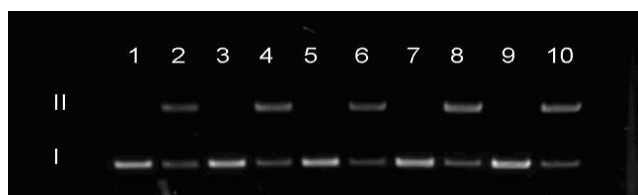
Figure 4-5 Thiol-dependent DNA cleavage by compound 4-1 . Assays were performed in 50 mM sodium phosphate buffer with different pH containing 0.5 \mu g of supercoiled pBR322 DNA in the presence or absence of compound 4-1 (50 \mu M) and 2-mercaptoethanol (250 \mu M). The total volume of reaction was 20 \mu L. The reaction time was 12 h. Lane 1/2, pH 6.0 without/with thiol; Lane 3/4, pH 6.5 without/with thiol; Lane 5/6, pH 7.0 without/with thiol; Lane 7/8, pH 7.5 without/with thiol; Lane 9/10, pH 8.0 without/with thiol.
