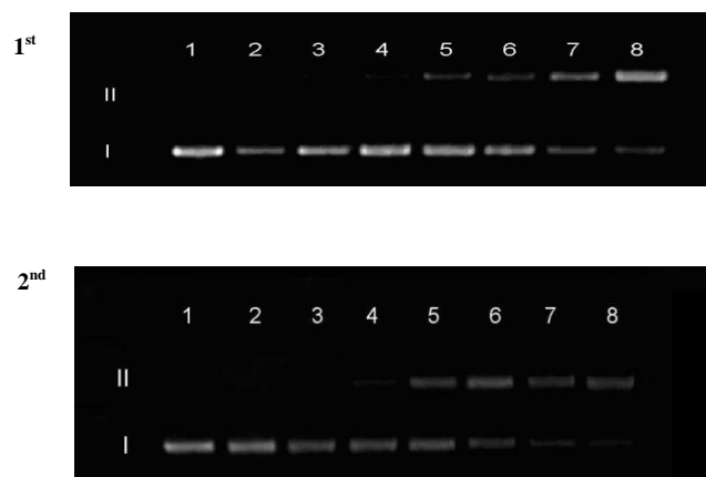
Figure 4-6 Time dependence of DNA cleavage by compound 4-1 (30 \mu\text{M} ). Assays were performed in 50 mM sodium phosphate buffer (pH 7.0) containing 0.5 \mu\text{g} of supercoiled pBR322 DNA in the presence or absence of compound 4-1 and 2-mercaptoethanol (total volume 20 \mu\text{L} ). The reaction times corresponding to lanes 2 to 8 were 2, 4, 6, 8, 10, 12, 24 hours, respectively.
