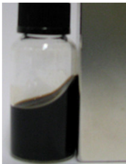
Figure 6.7. Photo of aqueous ferrofluid (in presence of a permanent magnet) consisting of magnetite nanoparticles prepared in TEG at 280°C.
