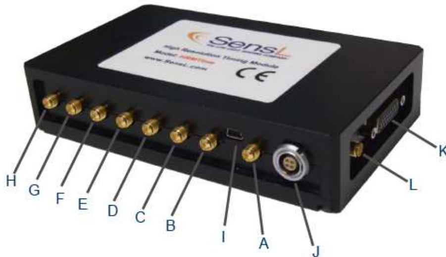
Figure 4.8 HRMTime Timing module from Sensl. A-H, Channel 0-3 Start&Stop Input (SMA TTL); I, USB connector; J, power supply connector; K, 16-way I/O port connector; L, Programmable Clock output (SMA TTL 50 ohm)
