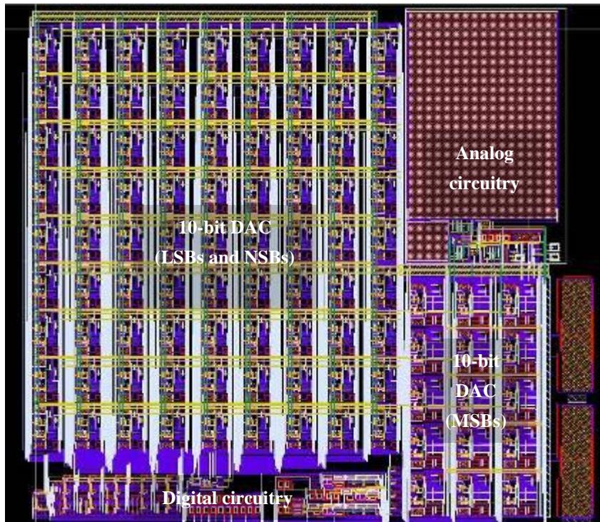
Fig. 7.15 Layout of the modified stimulator
