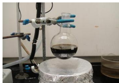
Silver nanoparticle ink after reduction
