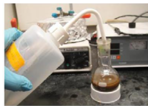
Ethanol was added to precipitate the nanoparticles and remove the unreacted oleylamine
