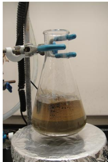
Ag Ink obtained after the addition of NaBH 4
