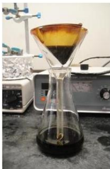
The organic layer was filtered to remove any undissolved impurities
