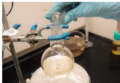
NaBH 4 was added into the mixture
