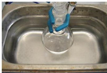
Ag NO 3 + Oleylamine+ Toluene mixture was sonicated until Ag NO 3 dissolved
