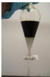
Aqueous layer was separated
