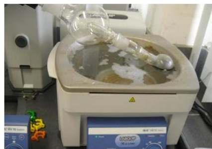
The toluene was fully evaporated from the filtered solution
