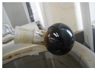
Toluene was fully removed to measured the weight of the particles
