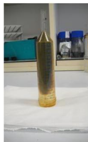
Nanoparticle precipitate after remove the ethanol and unreacted oleylamine
