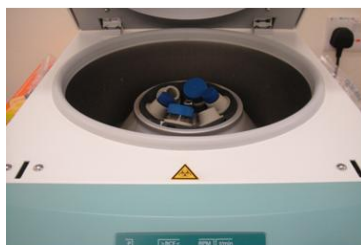
The Ag ink was centrifuged to concentrate the Ink
