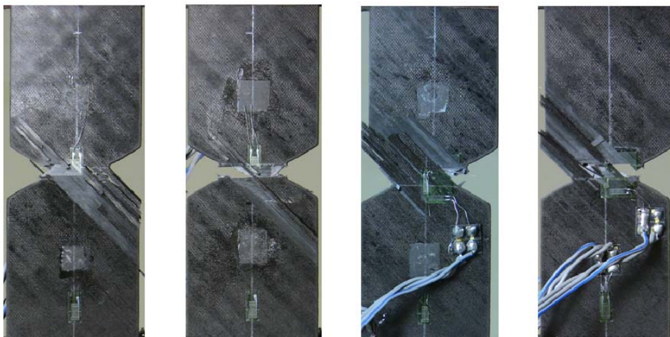
Figure 6-3 Failure of the notch-size scaled specimens after testing.
