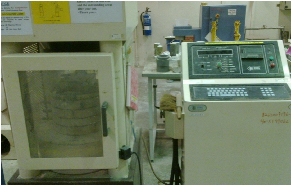
Figure 3.5 - Denison-Mayes compression test machine
