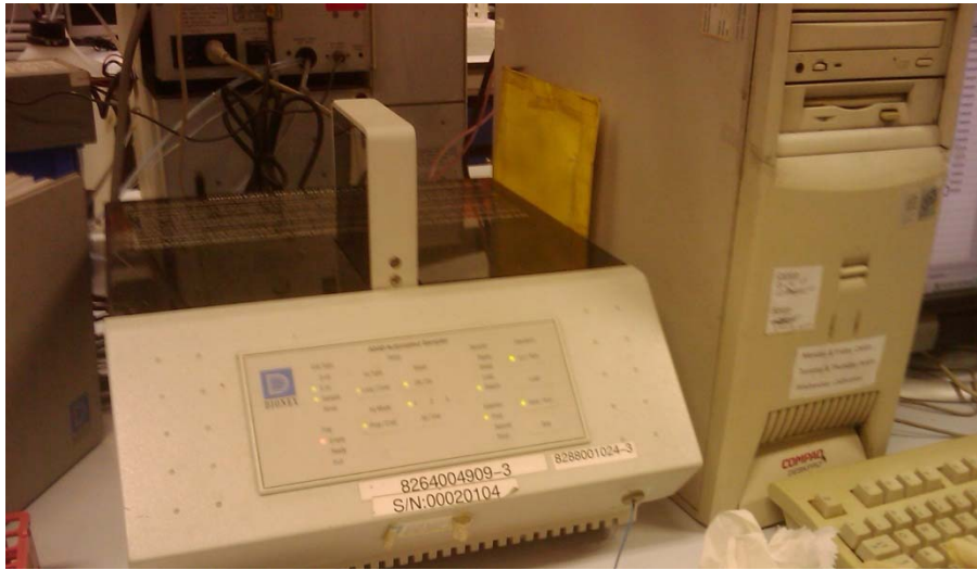
Figure 3 - 3 Ion chromatography system with auto-sampler for measurement of nitrate concentration
