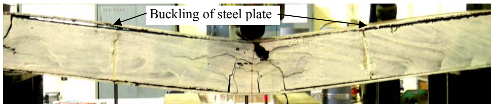
(e) Top plate buckling failure (beam SLCS)
