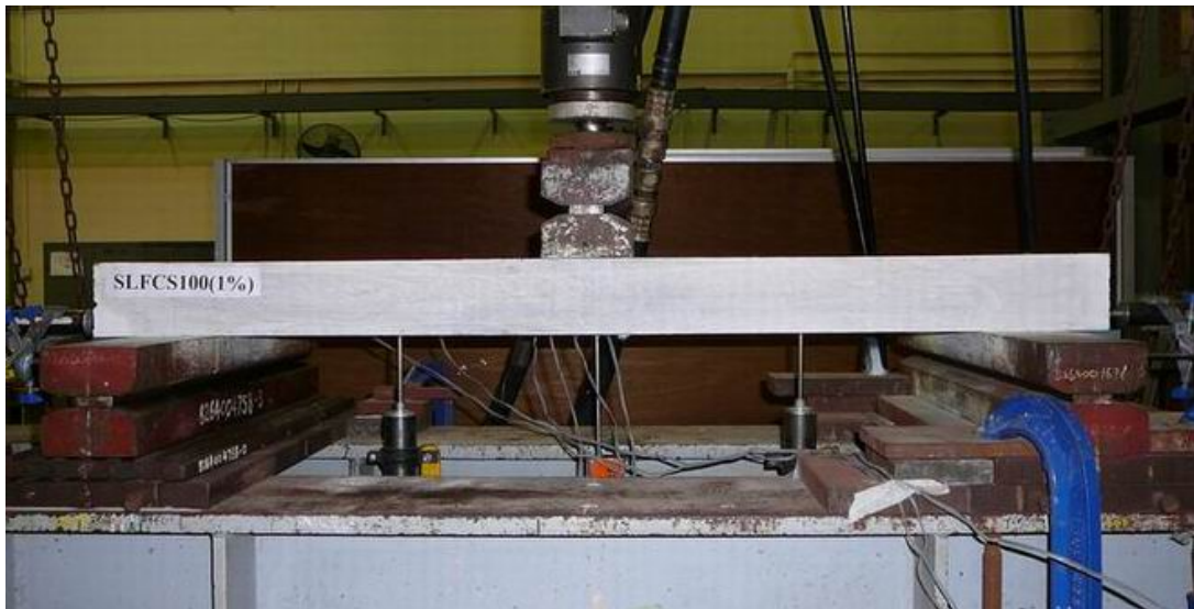
(b) Test set-up for sandwich beam specimen
