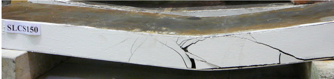
(b) Concrete shear failure
