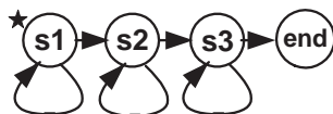
Figure 4.2: State transition diagram of an example HMM phone model with three states. Initial state probabilities are zero for all but the s1 state. Thus only the s1 state can be joined to states of the previous phone model when they are chained together in the HMM recognition model. The end state is not an actual state, it just identifies which state of this model (in this case only the s3 state) can be joined to states of the next phone in the recognition model (see text for explanation).
