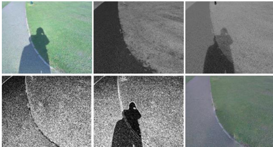
Figure 3.16: The shadow removal algorithm of [36, 37]. Top row: Original RGB image (left). Grayscale illumination invariant (middle). Grayscale normal (right). Bottom row: Edge map of illumination-invariant image (left). Edge map of normal grayscale (middle). Final shadowless RGB image (right).
