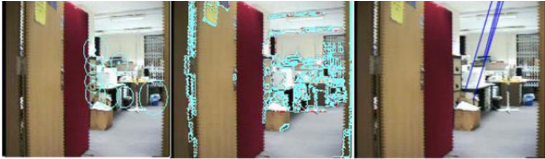
Figure 2.1: Solution from [87]. Kadir-Brady salient regions (left), MSER (middle) and SIFT descriptors (right).
