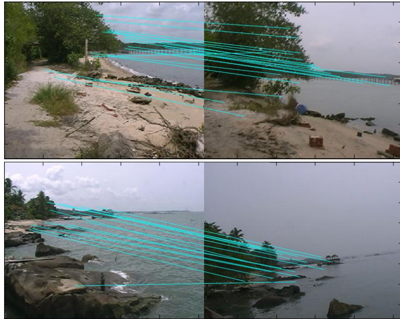
Figure 7.5: Challenging UBIN test scenes with significant image distortion - viewpoint, weather and illumination changes.
