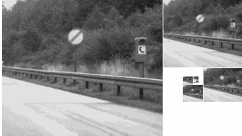
Figure 4.6: Image pyramids of the intensity composite feature maps formed by the repeated application of the \downarrow 2 operator and convolution with a Gaussian.
