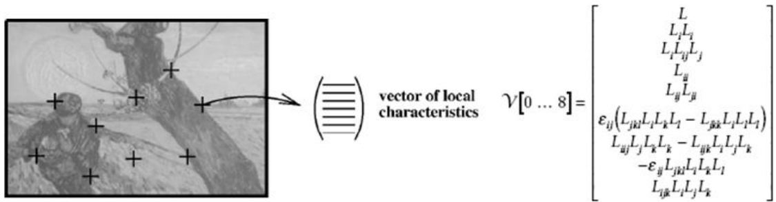
Figure 3.8: A vector of local characteristics is used to represent the detected interest points (keypoints) on an image (denoted by ‘+’) (left). The authors used a set of local differential invariants to compute the descriptors, summarised as a vector of ‘local jets’ (right). Adapted from [98].
