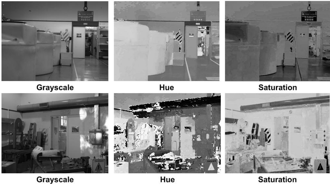
Figure 7.9: Two IND scenes with their HSV components. Comparing the grayscale images vs. the hue images reveals the strong dissimilarity between the two colour spaces. On the other hand, saturation images bear a stronger resemblance to grayscale.
