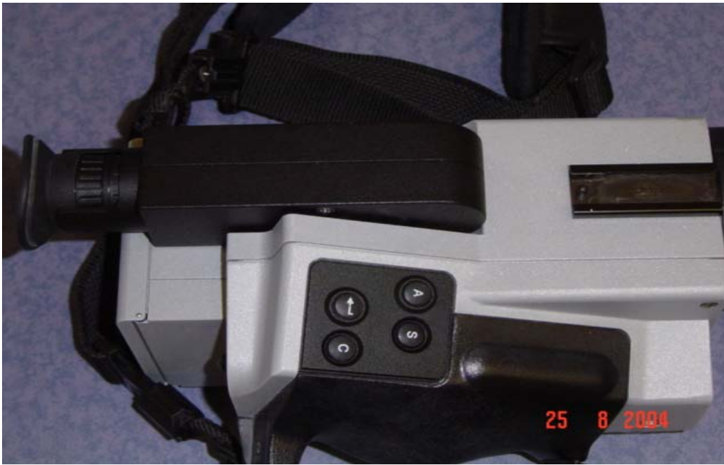
Fig 4: ThermaCAM™ PM575, infrared camera used for taking pictures of the dorsum of the hands.
