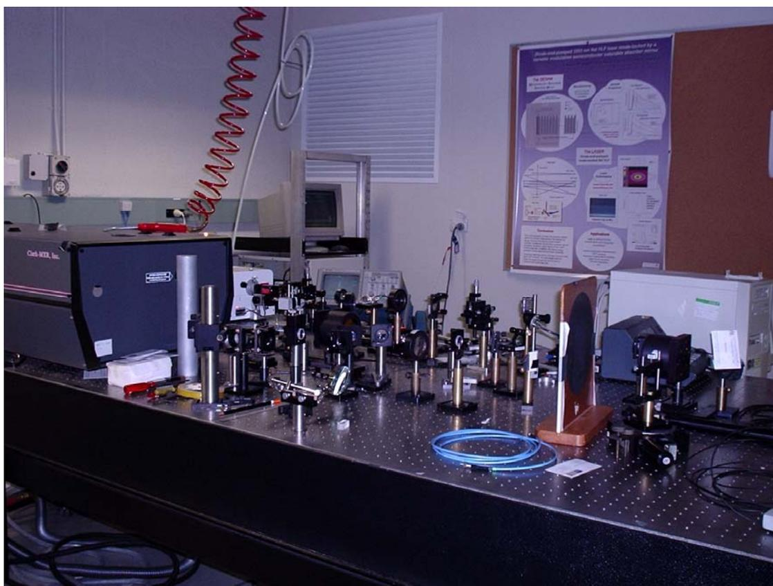
Fig. 3.3 Picture of the Z-scan setup at the Laser Physics Centre, The Australian National University, Canberra
