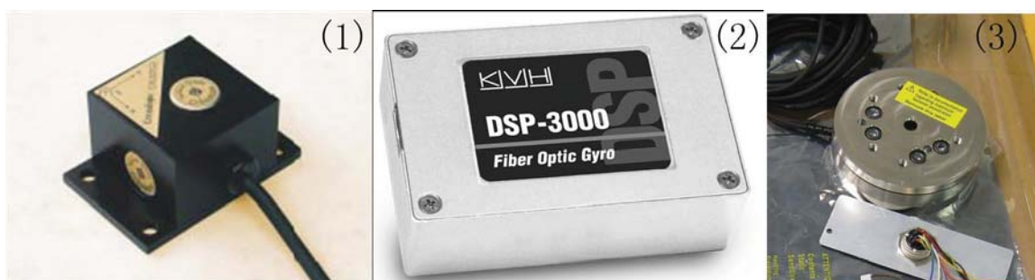
Figure A.9: Other sensors of ASLAN (1): accelerometer, (2) gyro, (3) force/torque sensor
