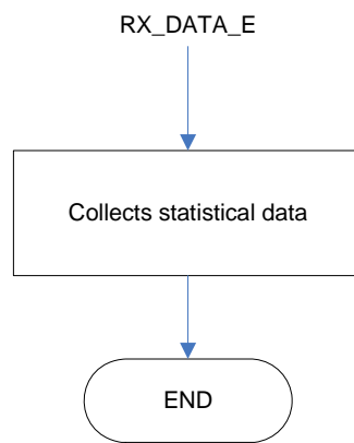
Figure D4: Flowchart of how the node reacts when the data segment is received.
