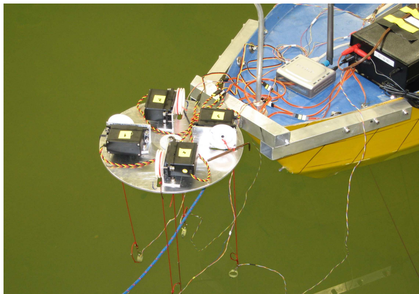
Figure 3.22. Close-up view of turret with 4 sail winches
