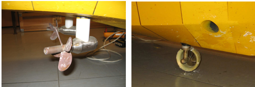
Figure A.6. Two aft azimuth thrusters (left), 1 fore azimuth thruster and 1 fore tunnel thruster (right) of Cybership III
