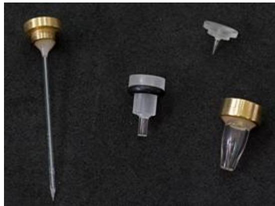
Fig. 3.8: Inkjet printhead nozzles fabricated from glass tube.
