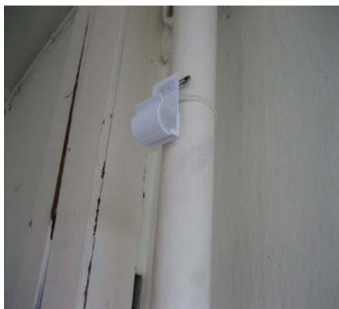
Figure 3.23 Ogawa PS-100 Passive Sampler at the 10 th Floor Outdoor Corridor in Front of Unit of #XX-268 at Block 401 (Case Study 4)
