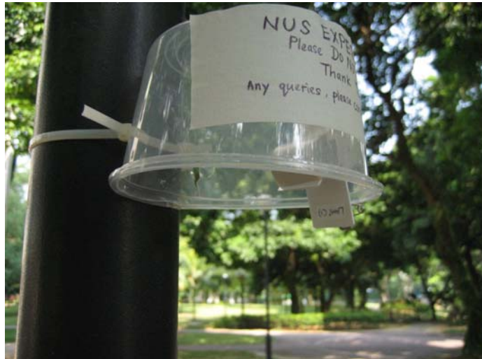
Figure 3.19 Ogawa Samplers strapped to Lamp Post in Front of Block 39 (Case Study 4)
