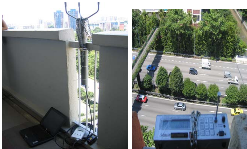
Figure 3.17 Instruments at the Low Floor Outdoor Balcony of Block 96 (Case Study 1)
