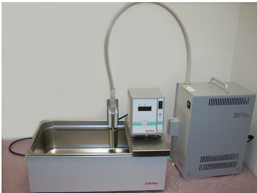
Figure 3.3: The apparatus used for experimental cold pain induction, consisting of a heating circulator with open bath and an immersion cooler.
