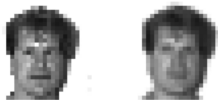
(a) Nearest neighbor algorithm, scaling quality 10. (b) Pixel area relation algorithm, scaling quality 10.
