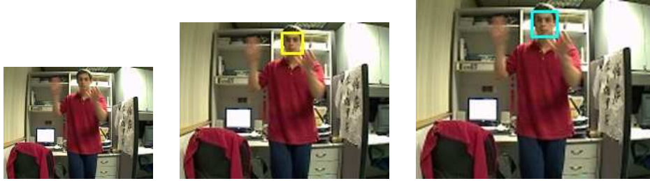
Figure 4.7: Examples of Viola-Jones detection for different resolutions of the practical video.
