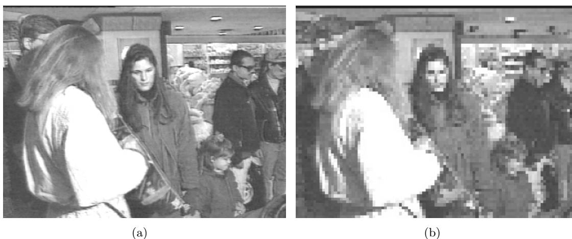
Figure 4.11: The effect of image down-scaling (to 30%) followed up by its up-scaling to original size. The image is from MIT/CMU dataset. Nearest neighbor scaling is used.
