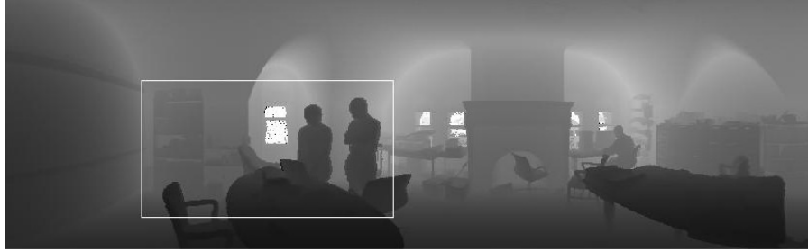
Figure 6.1: An office scene used. Intensity represents depth with distant object looking brighter. Regions with no range data appears black. The image plane of camera 1 is denoted by a white rectangle.
